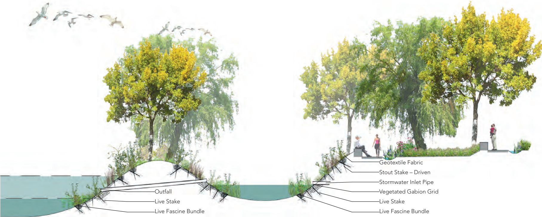
Ravine Section – Live Staking Bank Stabilizations
